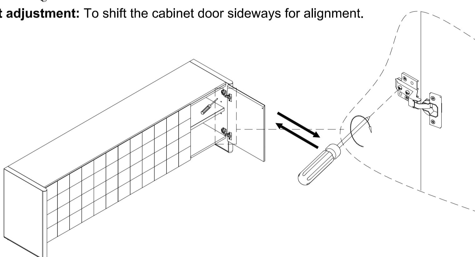
**3. Back and forth adjustment:** To move the cabinet door closer to or farther from the cabinet frame.
