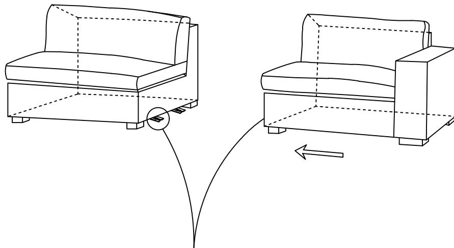
The prong and the connector must be aligned well.
