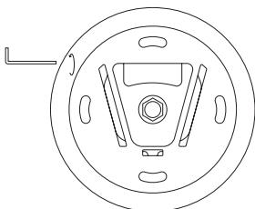
Use the included Allen key to unscrew the small lock screw on the ceiling plate.
