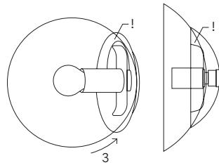
Slide the globe up so that the opening catches the bottom clamp.
