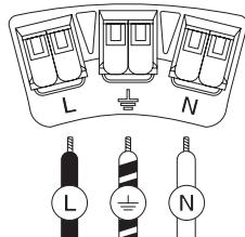
Use the included terminals to connect the wires and place the terminal holder flat in the ceiling plate.
