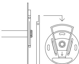
Slide the fixture plate into the ceiling plate as in the picture. Make sure no wires are squeezed.
