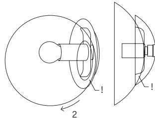
Move the globe slightly down to make sure the opening slides over the bottom clamp.
