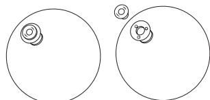
Start mounting glass globe from the top arm downwards by first removing the plastic stopper from the globe to be mounted.
