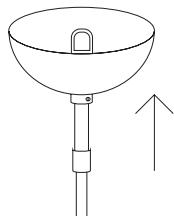
Lift the canopy [A] up and tighten the locking screw to hold the lamp in position.
