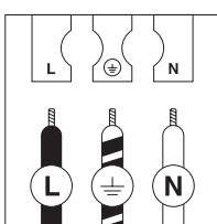
Junction boxes may vary depending on location. The diagram on the left shows the most common markings and manner of connecting the cords.
