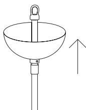
Lift the fixture up and hang it on the hook to make electrical connections.
