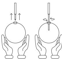
Carefully mount the globe onto the arm tip and screw it on.
