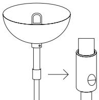
Loosen the line screw [D] and carefully pull/push the line to your desired length. Tighten the screw to secure the position. Excess line should be coiled inside the canopy.
