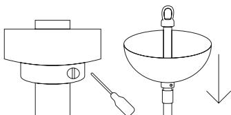
After removing the lamp from the box, use a flat-head screwdriver to loosen the locking screw [C] and lower the canopy [A].
