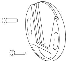
Place the plate against the ceiling/wall, depending on where the fixture is mounted, mark spots for anchors and drill the holes. Mount the plate to the ceiling/wall.
