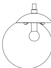
Place the globe opening on one of the clamps and slide it on as far as possible. Repeat the same movement for one more clamp.
