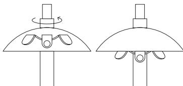
To start mounting the glass globes, turn the cap on the selected arm counterclockwise until it stops.
