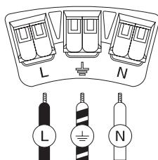
Use the included terminals to connect the wires and place the terminal holder flat in the ceiling plate.
