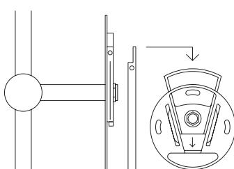
Slide the fixture plate into the ceiling plate as in the picture. Make sure no wires are squeezed.
