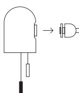
Place the smaller outer ring [F] onto the socket and screw the retainer ring [D] onto the socket to secure the glass cylinder. The inner and outer rings let you set the cylinder in the right position.
