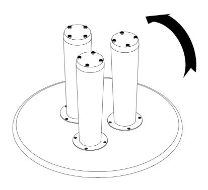
CAUTION – TAKE EXTREME CARE WHEN TURNING TABLE ATER ASSEMBLY, DO NOT USE LEGS AS PIVOT.THIS WILL CAUSE IRREPARABLE DAMAGE TO JOINTS.
