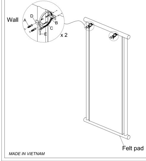
REMARK: There is a tip restraint kit provided on the back of this product please read the direction thoroughly and install immediately
