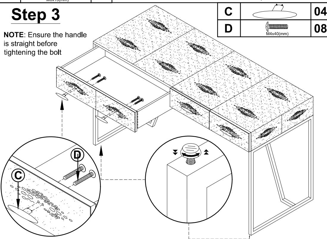
NOTE: Ensure the handle is straight before tightening the bolt
